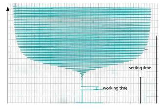
The Speedex rheology diagram clearly shows a "steep" snap set characteristic.
